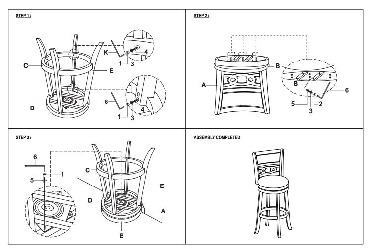
DO NOT TIGHTEN BOLTS UNTIL COMPLETELY ASSEMBLED
